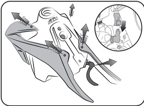
**1. Remove the radiator scoops. Disconnect the fuel pump cover cable and the fuel connector as indicated in the diagram.**
