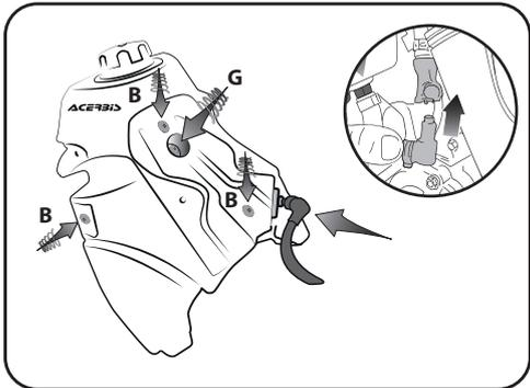
**4. Place the Acerbis fuel tank (A) on the bike. Insert the tank and seat screws (G/B) as indicated in the diagram. Reconnect the fuel pump power cable and the fuel connector.**
