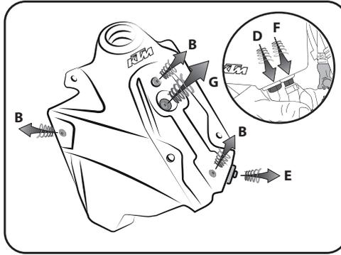
**2. Remove seat screw (B) and the screws on the side. Remove the tank screw (G), then empty any remaining fuel from the tank. Remove the (D/E/F) fasteners and remove the fuel pump.**
