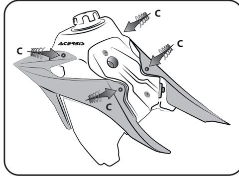
**5. Assemble the radiator scoops with the screws (C).**
