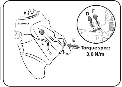
**3. On the fuel tank Acerbis (A), reconnect the fuel pump (E) with the original screws/hardware.**
